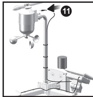
11. Plug the other solar panel cables into the socket on the wind vane.
