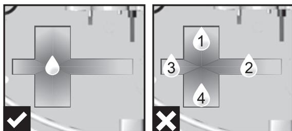
Water will pool to the center of the cross when the rain gauge is level.
