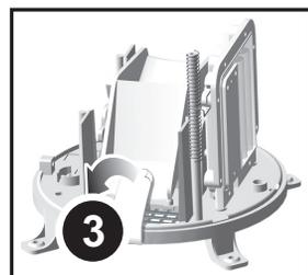
3. Remove the fibre tape.
