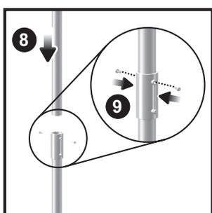
6. Assemble middle pole on top of the bottom one.
