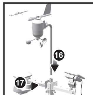
16. Insert the wind vane into the attachment bracket.
