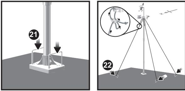
21. Insert the 2 rectangular base legs through the holes of the versatile base and hammer down.
