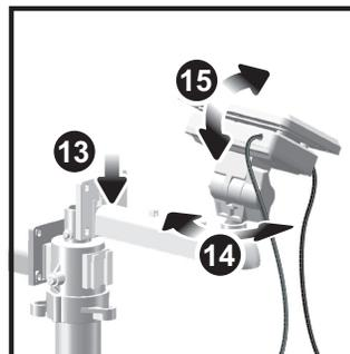
13. Slide the solar panel connector into place on the opposite side of the bracket. Slot the solar panel in place.
