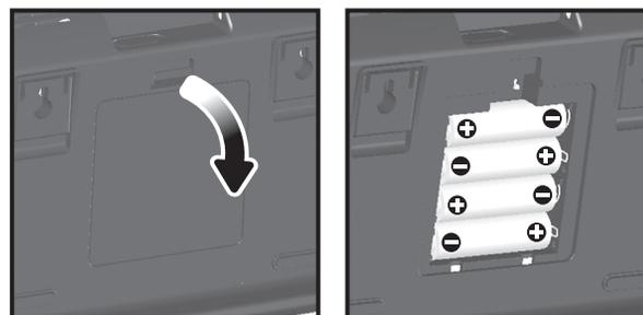
Install the base station batteries (4 x UM-3 / AA) matching the polarity (+ / -). Press **RESET** after each battery change.
