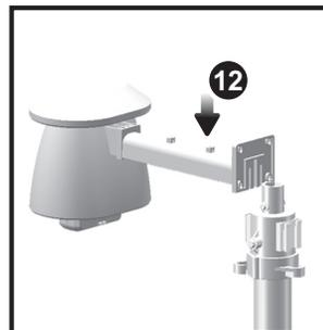
12. Slide outdoor sensor onto vertical attachment bracket.
