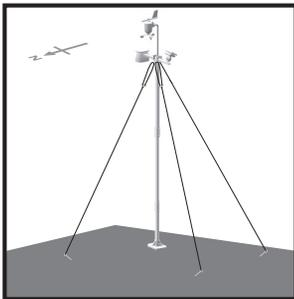
**ALTERNATIVE SET UP: REMOTE WIND SENSOR ON EXISTING POLE**
