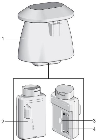
4. Insert sensor into the casing, twist and click to the right to secure.
