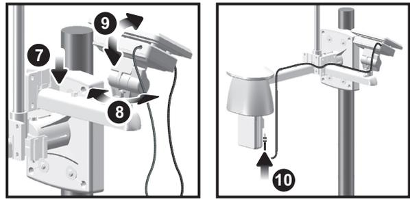
7. Slide the solar panel connector into place on the other side of the bracket. Slot the solar panel in place.
