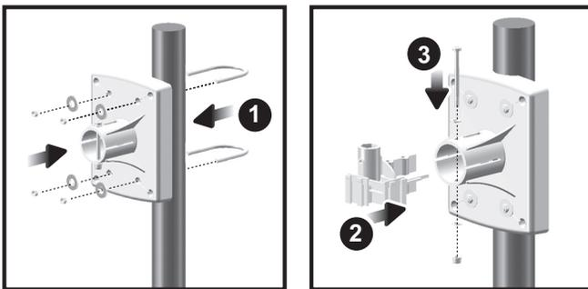
1. Secure the plastic base onto existing pole with U-bolts, washers and bolts.
