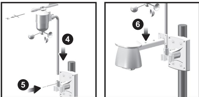
4. Insert wind sensor into the top of the bracket.
