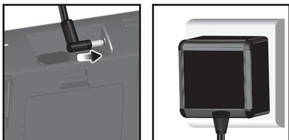
For continuous use, install the AC adapter. The batteries are for back-up use only.
