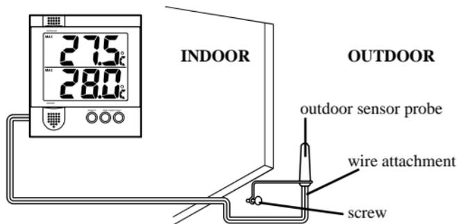
**Note:** Locate the outdoor sensor probe away from direct sun light and heavy precipitation.
