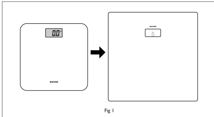
1. Observing the above caution, choose a suitable location for the mirror unit ensuring the scale can be comfortably accessed. Allow sufficient space around the mirror unit for removing and replacing the scale (Fig 1). The scale may be removed or replaced from either side.
