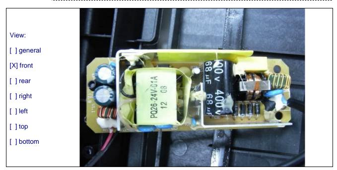
Details of: Switching power PCB
