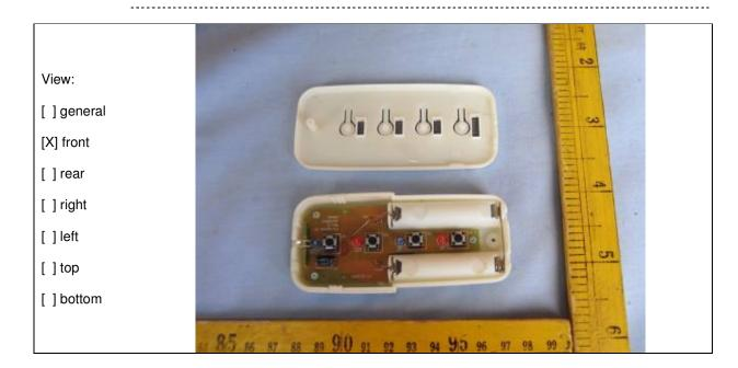
Details of: PCB for Remote controller
